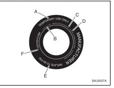
A. Temporary Use Only Marking The compact spare tire should not be driven at speeds over 50 mph (80 km/ h). The compact spare tire is for emergency use when a regular road tire has lost air and gone flat. See "Compact Spare Tire" and "If a Tire Goes Flat" in this section.
